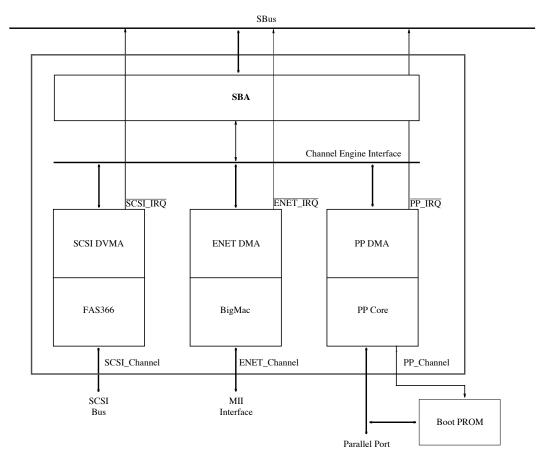
Figure 1. STP2002QFP Block Diagram
